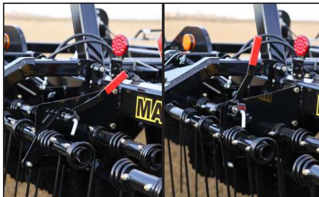
Fig. 57 Two Row Tine Harrows - Vertical Adjust/Angle Adjust
