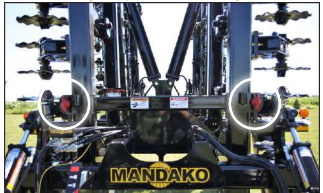
Fig. 27 Transport Lock Pins Installed
