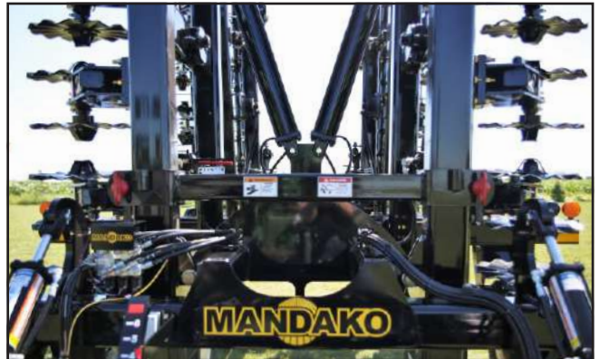
Fig. 66 Transport Lock Pins - Installed
