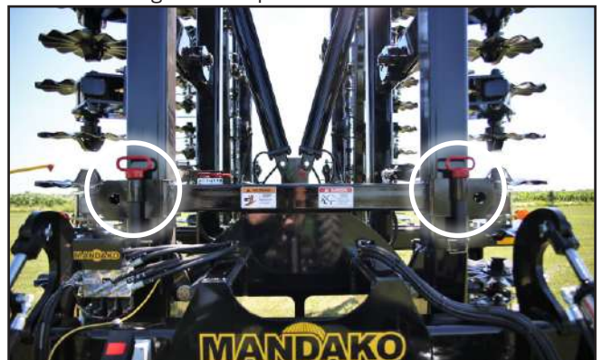
Fig. 28 Transport Lock Pins Removed and Stowed
