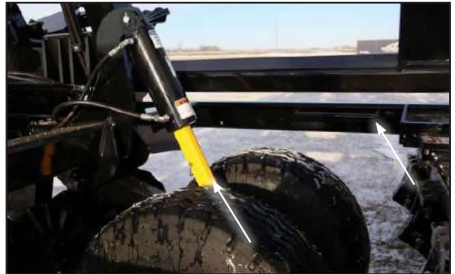
Fig. 26 Cylinder Stop and Storage
