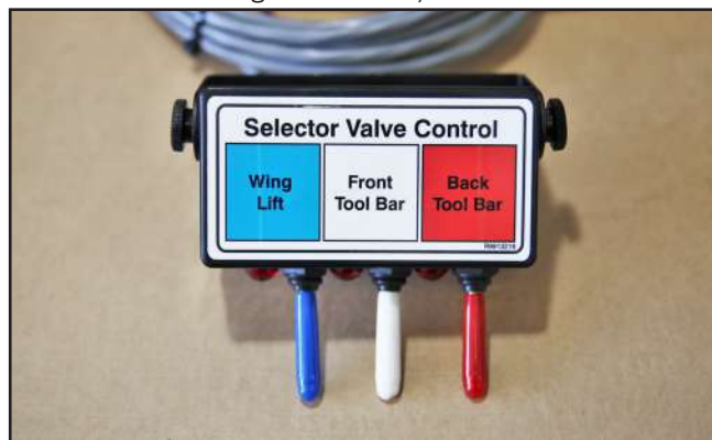
Fig. 22 Selector Valve Control Box
