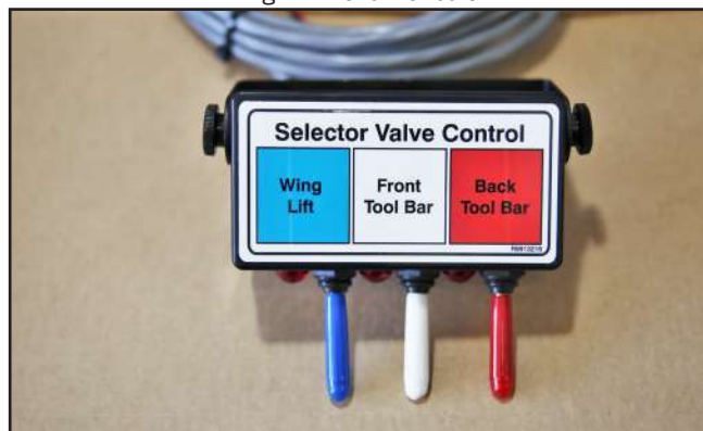
Fig. 28 Selector Valve Control Box
